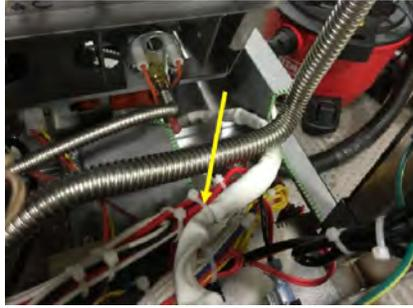
NOTE: When facing the front of the fryer, ensure the far right vat has wire tie radio cable secured to existing bundle as shown.
