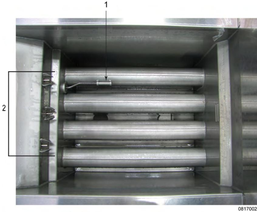
**Figure 7-3 Thermocouple & Probe Assembly**
